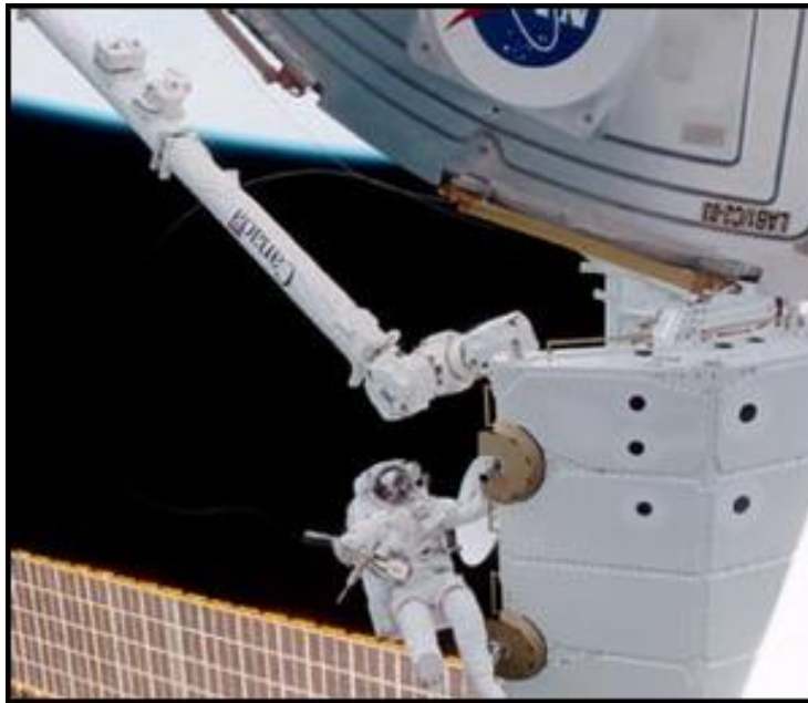
Figure 3: Completing an EVA activity using the robot arm with a crewmember on the end from inside the shuttle requires careful allocation of functions and task planning.
