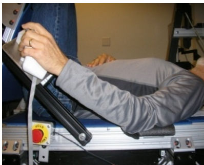
Figure 2. Cursor control device being tested in vibration chair.
